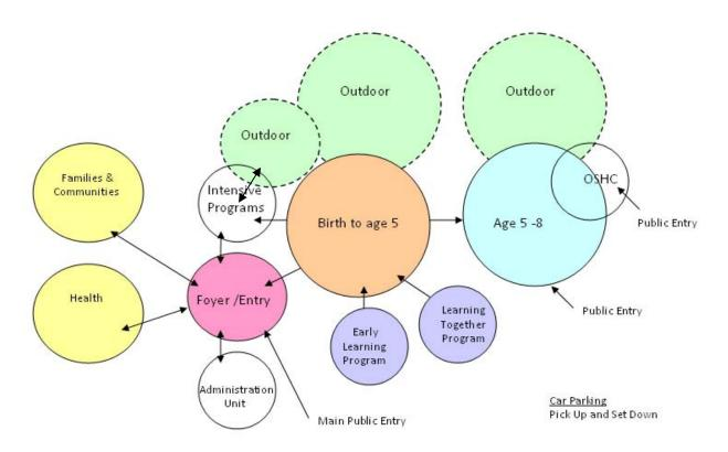
The site planning and building design of each project should consider the ability to add future modules, considering possible future site access points, the relationships between modules and circulation through the planned facility.
