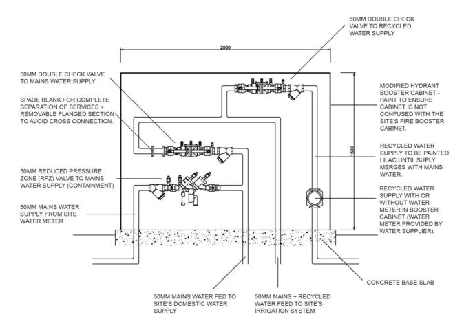
Option 2: separate housing – mains and recycled water connection cabinet
